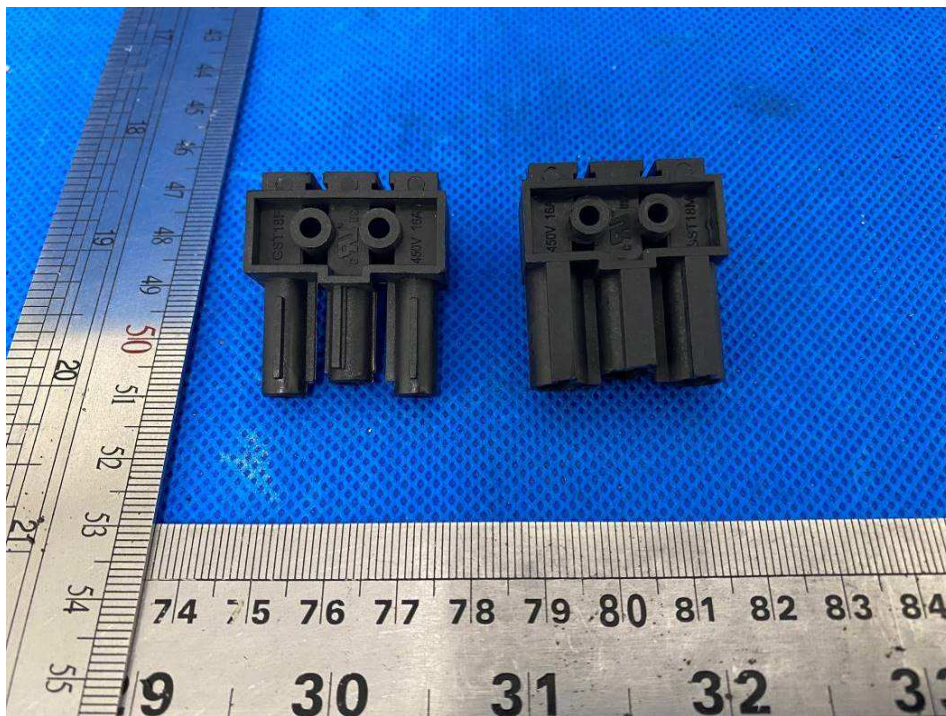
Figure 76: Terminal block view
