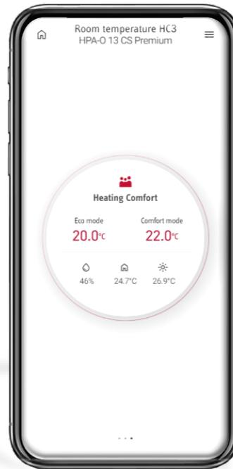
Temperatures can be adjusted in 0.5°C (short swipe) to 1°C (long swipe) increments. Hold to scroll.
