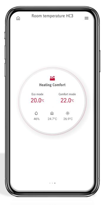
Temperatures can be adjusted in 0.5°c (short swipe) to 1°c (long swipe) increments. Hold to scroll.
