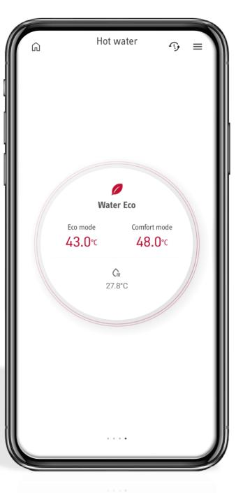
To adjust the comfort and eco temperature simply tap of the displayed temperature and enter your desired temperature.
